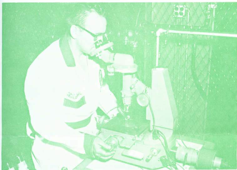
William F. Solocius examines a finished part under a special industrial toolmaker's microscope.
