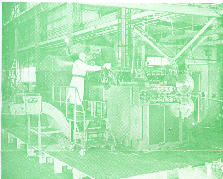
Farrelite Ralph W. O'Loskey starts a No. 5 Progressive header to test its tools designed to make automotive anchor pins.
